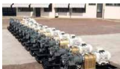
API685 Magnetic Drive Pumps for Oil&Gas Process
